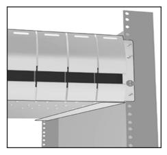
5. Snap the end cap over the screw on each side of the unit to finish the installation.
